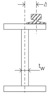
**9.6.16 Rail surface at joints in gantry crane rails**
