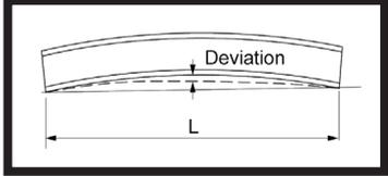
**7.3 PERMITTED DEVIATIONS FOR ELEMENTS OF FABRICATED COMPONENTS ( $\Delta$ )**
