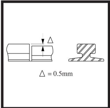
**9.6.17 Rail edge at joints in gantry crane rails**
